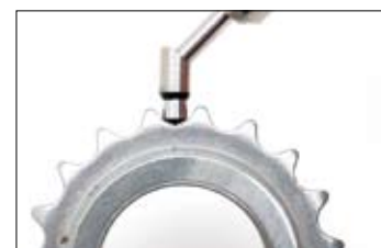
Micro-probes produce precise results even from hard-to-access areas.
