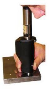
The small area of the nose piece allows indentations to be read close up to shoulders, in corners etc. where Brinell hardness testers can make them but where other microscopes cannot reach, such as on pulleys, sheaves etc. Consequently only a smaller surface area has to be prepared. When the piece to be tested has a convex or concave surface, the BRINscope Brinell Microscope measures more accurately, since the small base fits flush on the indentation.
