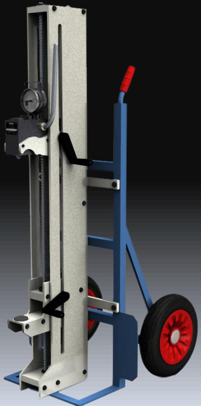
**Setting the standards in Brinell hardness testing equipment**
