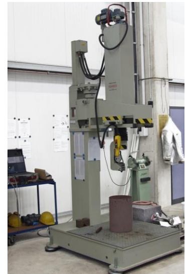
The BHD Type B is a higher specification machine using a multi-force closed loop (load cell controlled) servo motor controlled test head that includes automatic timing cycle. It offers indentation only and is ideal for use with an external Foundrax BRINscope manual or BRINtronic fully automatic Brinell microscope for indentation measurement.
