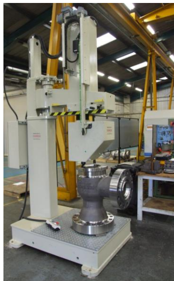
The BHD Type B is a higher specification machine using a multi-force closed loop (load cell controlled) servo motor controlled test head that includes automatic timing cycle. It offers indentation only and is ideal for use with an external Foundrax BRINscope manual or BRINtronic fully automatic Brinell microscope for indentation measurement.
