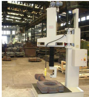
The BHD Type B is a higher specification machine using a multi-force closed loop (load cell controlled) servo motor controlled test head that includes automatic timing cycle. It offers indentation only and is ideal for use with an external Foundrax BRINscope manual or BRINtronic fully automatic Brinell microscope for indentation measurement.
